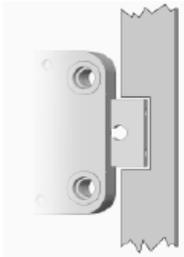
In the LOCKED position, there should be approximately 1 mm clearance between the lock bolt and the cavity in the blocking bar of the boltwork. The lock bolt must move freely into the cavity.
