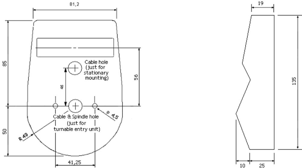
With mounting plate add 3mm to thickness; with turnable plate add 9,7mm.
