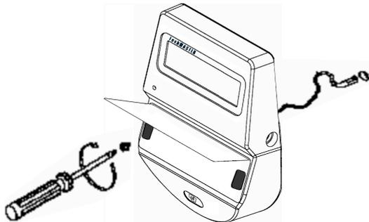
Remove the protective film from the membrane, carefully align the margins and stick it to the housing.
