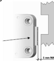
Any component attached to the bolt must be approved by Tecnosicurezza before installation. Only use supplied screws to mount the lock. Tighten the screws securely so the lock body is attached firmly to the mounting surface (Torque approximately 10 Nm). To avoid damage to the cable, the hole should be completely seated.
