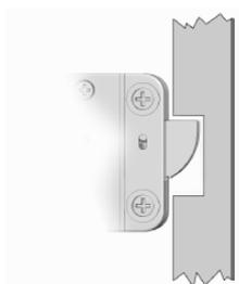
In the LOCKED position, there should be approximately 1mm clearance between the lock bolt and the cavity in the blocking bar of the boltwork.
