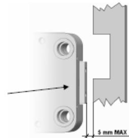
The force applied to the bolt must not exceed 1kN. Any component fixed to the bolt must be approved before the installation.
